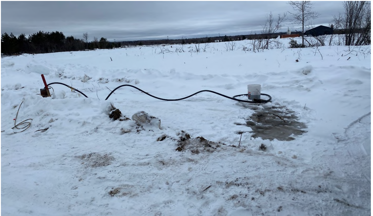
Photo 2: General view of pumping test set-up for Test Well No. 2. (Tetra Tech, January 2022)
